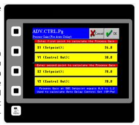
Note: In cases where the set point has been changed or if the feeder is run with no product and the valve opens to 100% open, upon restart, the new valve position will be calculated as mentioned above. Otherwise, the Auto Delay will retain the last known good valve position.
